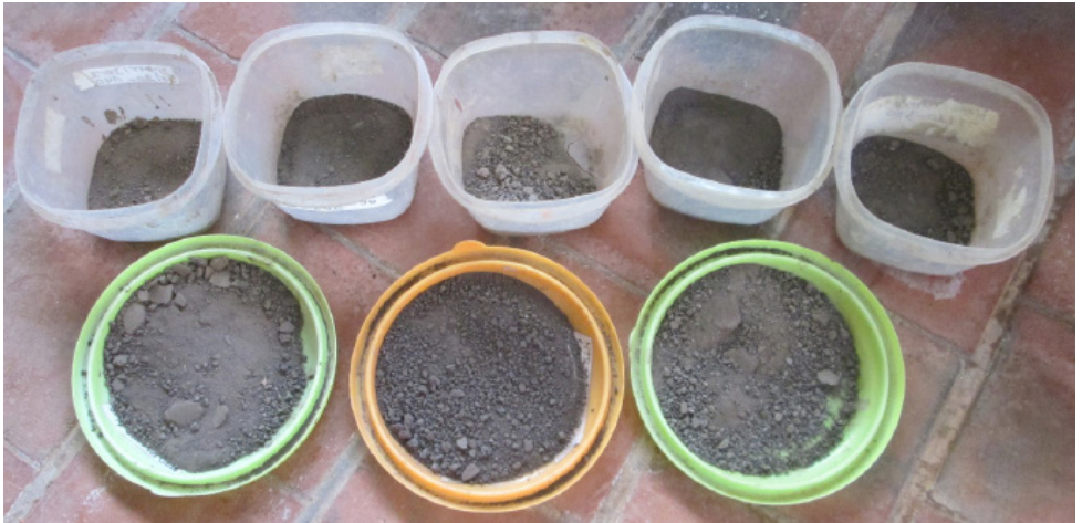
dried soil samples and grinded ones for hydrometer analysis (specimen 2)
