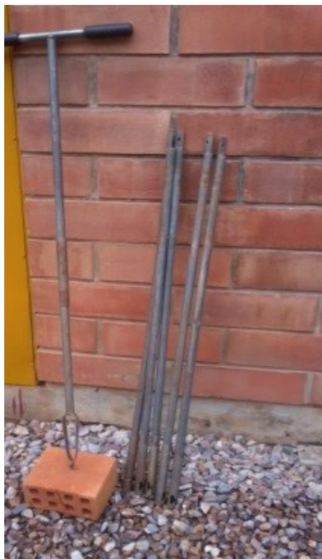
Soil auger: Tool for soil drilling and sampling activities
