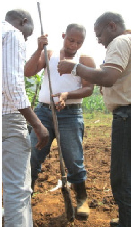
Soil sampling and samples recuperation from the field
